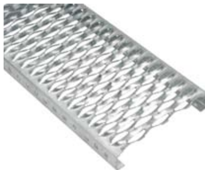
Type AP 1.5-30/SER (1.5 mm sheet) Type AP 2-30/SER (2 mm sheet) Type AP 2.5-30/SER (2.5 mm sheet) Anti-slip perforation 13 mm, c.t.c. 27 mm, 10 mm high.
