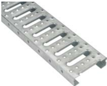
Type AP 1.5-30/STE (1.5 mm sheet) Type AP 2-30/STE (2 mm sheet) Type AP 2.5-30/STE (2.5 mm sheet) Anti-slip perforation Ø 8 mm, c.t.c. 60 mm, 2 mm high.
