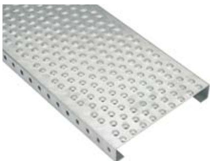
Type AP 1.5-30/GES (1.5 mm sheet) Type AP 2-30/GES (2 mm sheet) Type AP 2.5-30/GES (2.5 mm sheet) Anti-slip perforation Ø 15 mm not fully punched out, c.t.c. 20/40 mm, 3 mm high. Perforation pattern; 2 equal rows followed by 1 row, staggered.
