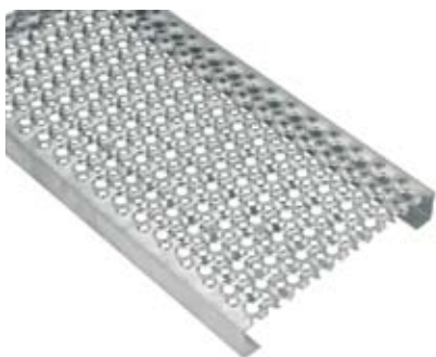
Type AP 1.5-30/RUN (1.5 mm sheet) Type AP 2-30/RUN (2 mm sheet) Type AP 2.5-30/RUN (2.5 mm sheet) Anti-slip perforation 2x Ø 8 mm, c.t.c. 15/30 mm, 2 mm high. Drainage perforation Ø 11 mm, c.t.c. 15/30 mm, 3 mm deep.
