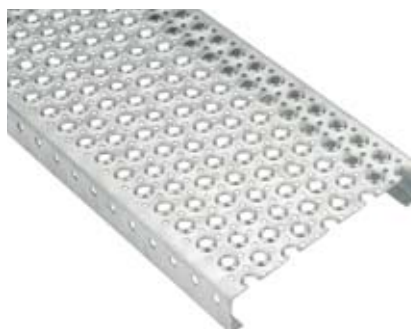
Type AP 1.5-30/OFF (1.5 mm sheet) Type AP 2-30/OFF (2 mm sheet) Type AP 2.5-30/OFF (2.5 mm sheet) Anti-slip perforation Ø 11 mm, c.t.c. 15/30 mm, 2 mm high. Drainage perforation 2 x Ø 6 mm, c.t.c. 15/30 mm, 0 mm deep.
